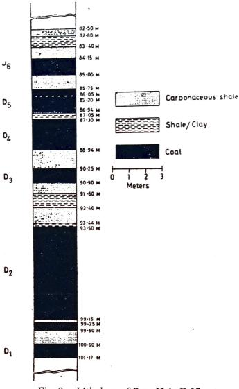
Fig. 2. Lithology of Bore Hole D 97
