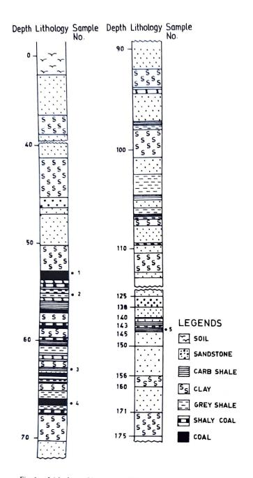
Fig 1. Litholog of bore core SGG-1
