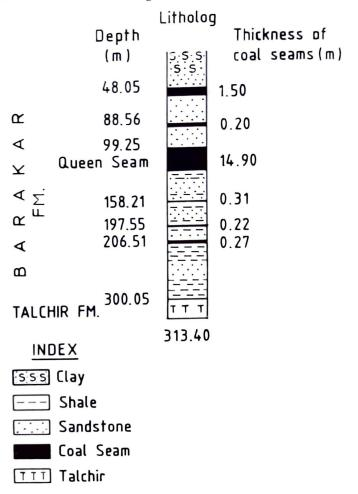
Fig 1.Litholog of bore core GKY-1 showing position of coal seams
