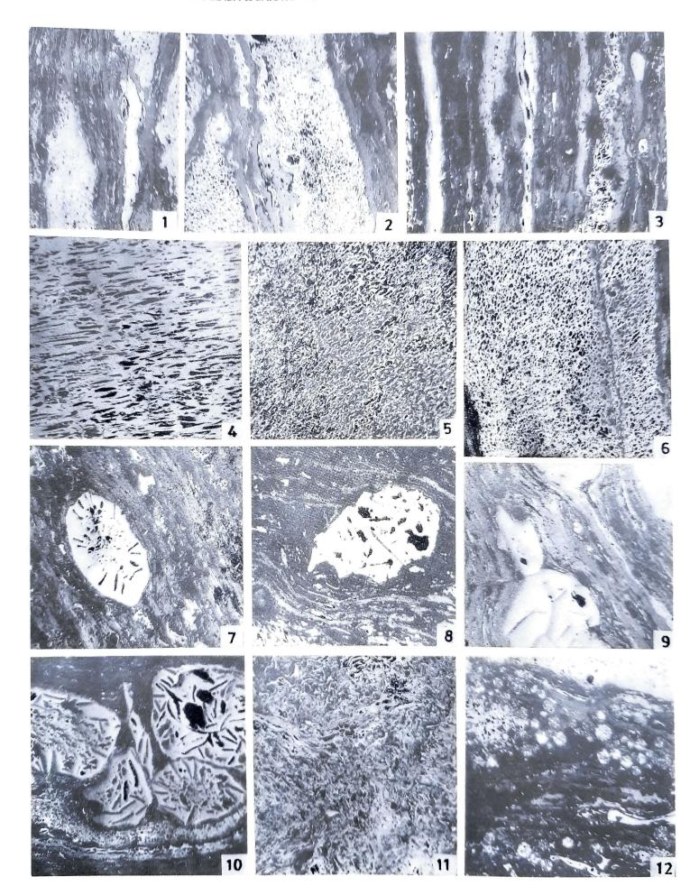
closer resemblance with Bagdona seam of PK-I Incline. The middle part of the seam is of better quality, as it contains only (19.6%) mineral matter. Whereas, the mineral matter is present in higher amount at upper and lower parts of the seam. Inertinite has a percentage distribution of (15%-20.8%).
