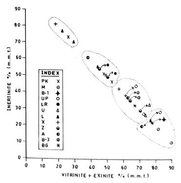
Text-figure 3. Showing different coal types present in Pathakhera Coalfield.
