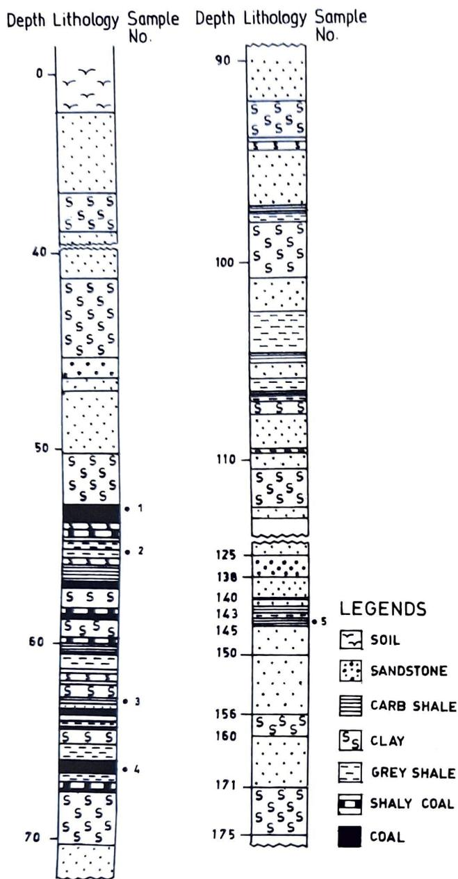
Fig 1. Litholog of bore core SGG-1
