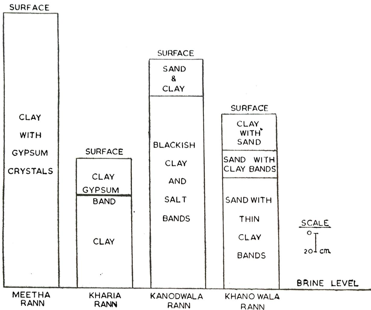
Fig. 1.—Profiles showing the nature of the sediments.
